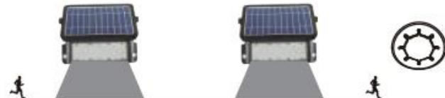
After activation, the floodlight automatically lights up to 20% of its maximum power for the entire duration.
