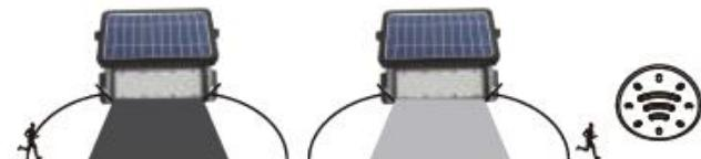
When the motion is detected (up to 8m), the floodlight automatically lights up with full (100%) power, then after 20 seconds of no motion detection, the light power value switches to 3% of the maximum value.
