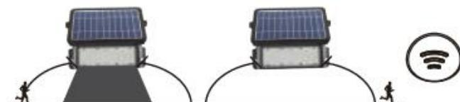
When motion is detected (up to 8m), the floodlight automatically lights up with full (100%) power, then turns off the lighting source after 30 seconds of no motion detection.
